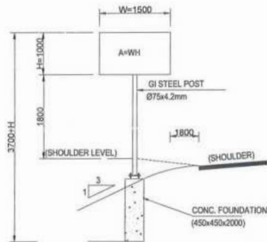
2 SINGLE POST (A<1.5m.) 2< FOUNDATION TYPE-1
