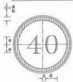
SPEED LIMIT SIGN R-25-4 DIMENSIONS (cm)
