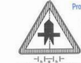
MINOR ROAD CROSSING AT RIGHT ANGLE W-27
