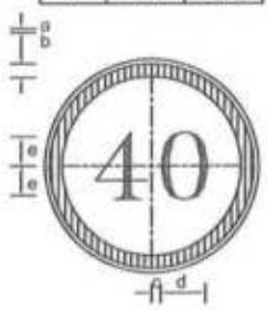
SPEED LIMIT SIGN R-25-4 DIMENSIONS (cm)
