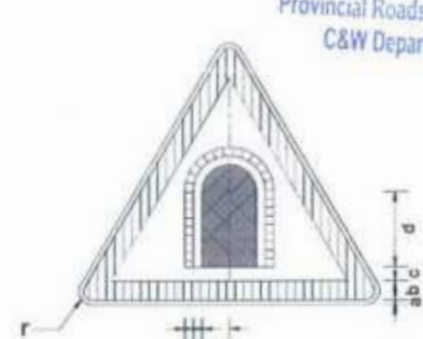
TUNNEL SIGN W-40
