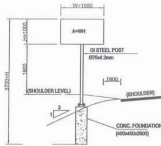
2 SINGLE POST (A < 1.5m.) 2 < FOUNDATION TYPE-1
