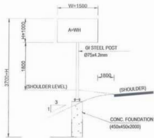
2 SINGLE POST (A<1.5m.) 2< FOUNDATION TYPE-1
