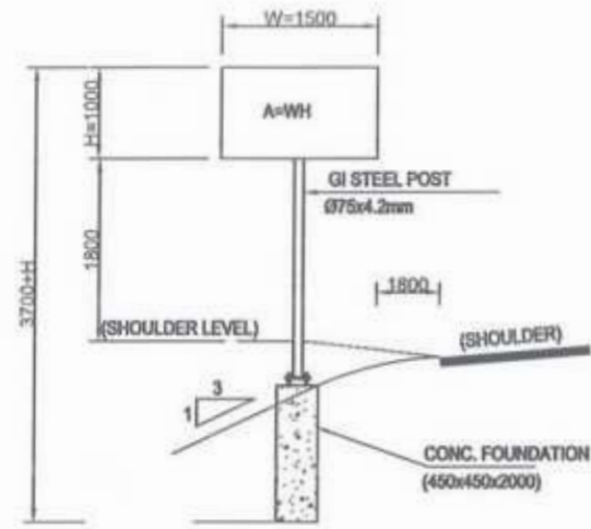
2 SINGLE POST (A < 1.5m.) 2 < FOUNDATION TYPE-1
