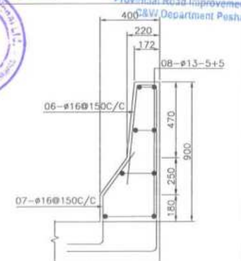
BARRIER REINFORCEMENT
