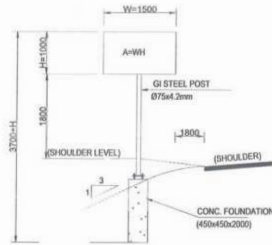
2 SINGLE POST (A<1.5m.) 2< FOUNDATION TYPE-1
